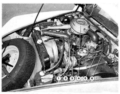
1, hydraulic fluid reservoir. 2, radiator filler cap. 3, distributor. 4, air cleaner. 5, dipstick. 6, coil.
