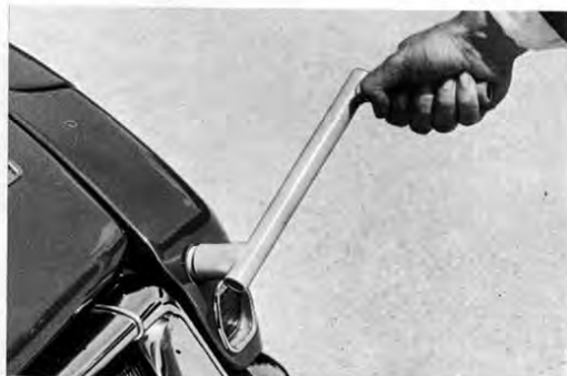
Fig. 32 - Removal of a rear wing
