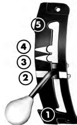
Fig. 16 - Ground clearance adjustment 1 - Minimum height 2 - Normal running height 3-4 - Special heights 5 - Maximum height
