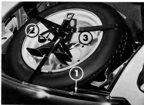
Fig. 31 - Tools for removing wheels 1 - Joint starting handle and wheel brace 2 - Stay 3 - Peg
