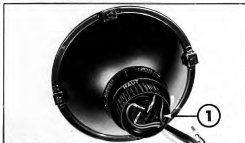
Fig. 38 - Main beam/Dipped (large diameter) Cibié European-Dip type bulbs (if fitted) 1 - Sidelamp (see page 33)
