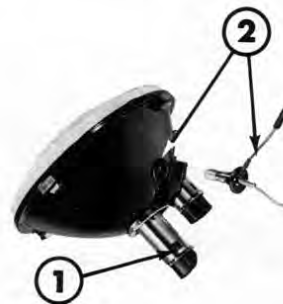
Fig. 40 a - Main beam/Dipped (large diameter) Cibié H 1 Quartz Iodine bulbs (if fitted) 1 - Release stop 2 - Sidelamp (see page 33)
