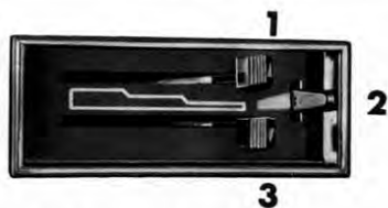
Fig. 22 - Side ventilators control 1 - Ventilation of upper interior 2 - Direction of ventilation of upper interior 3 - Ventilation of lower interior
