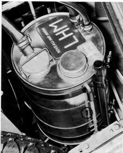
Fig. 26 - Hydraulic reservoir 1 - Level checking sight-tube
