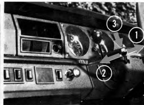
Fig. 20 - R.H.D. Manual gear-change - headlamp control 1 - 'Side and tail' or 'Main beam' positions 2 - Dipped position 3 - Directional headlamps
