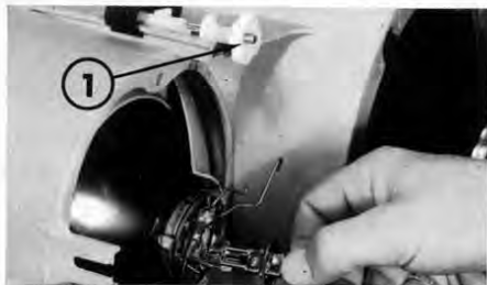
Fig. 46 - Long-range headlamps (small \varnothing ) directional 1 - Vertical adjuster
