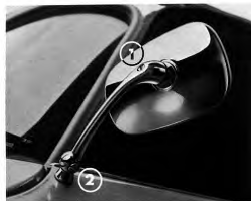
Fig. 9 - Outside rear-view mirror 1-2 - Adjusting screws
