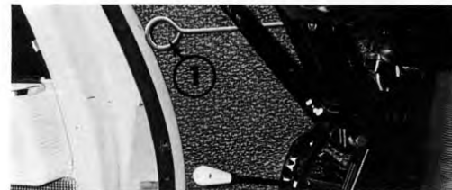
Fig. 3 - Opening the bonnet 1 - Unlocking ring
