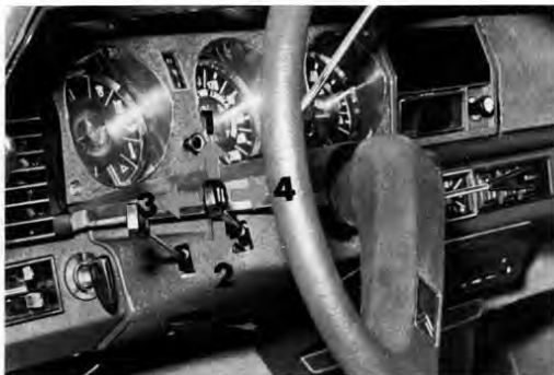
Fig. 18 - Signal switches 1 - R.H. indicators flasher 2 - L.H. indicators flasher 3 - Headlamp flasher 4 - Horns
