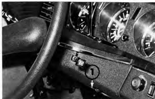
Fig. 12 - Starting with starting handle (on hydraulic gear-change version) 1 - Auxiliary clutch lever
