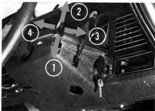
Fig. 18 - R.H.D. Manual gear-change signalling 1 - R.H. direction indicator 2 - L.H. direction indicator 3 - Headlamp flasher 4 - Horns
