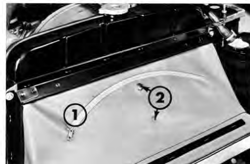
Fig. 29 - Cleaning the radiator 1 - Zip fastener 2 - Press stud
